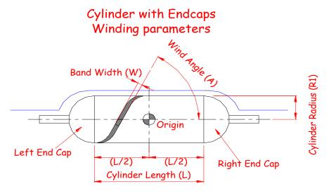
For each type of end cap other parameters **R2** and **R3** may be required. This depends in the endcap type and is described on the following page.
