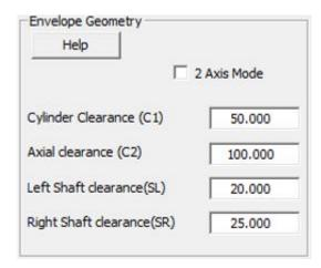
**SL** and **SR** are the left and right shaft clearance position measured from the winding shaft centre (axis). If there is no shaft zero can be used at one end. Set these values to as small as is safe for the machine and mandrel.
